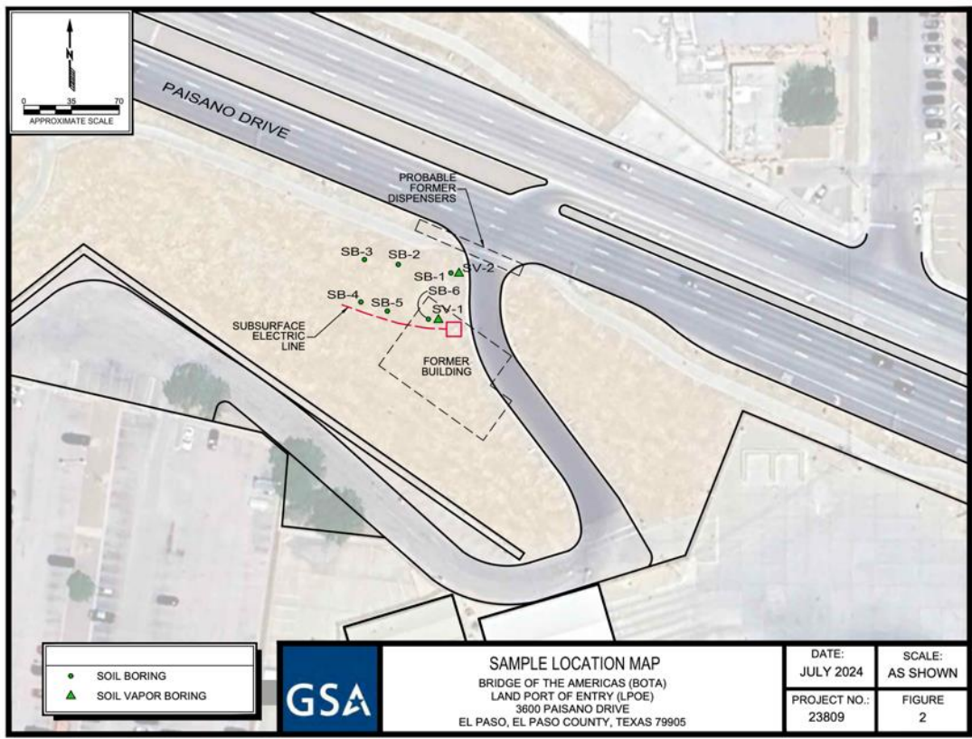
Figure 3-4. Location of Limited Phase II ESA Soil Borings.
