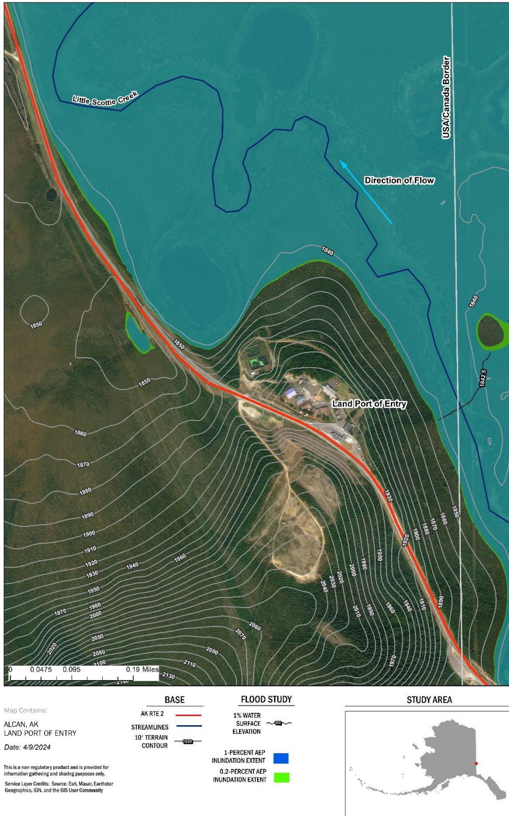
Figure 7. Local site inundation map
